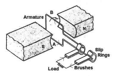
The diagram on the left represents a simple generator whose coil is being rotated clockwise (as seen from the slip rings). The coil has 156 loops, each formed from a square whose side length is 12.5cm. The magnetic field intensity is 0.324T and the coil / armature is being rotated at  $1.20 \times 10^3$  rpm. The external load has a resistance of  $2.58\Omega$ .
