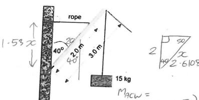
The diagram on the left shows a system in static equilibrium. The 3.00m long uniform beam has a mass of 12.5kg and supports a mass of 15.0kg from its end. It is hinged to the wall of a building, making an angle of 40.00 to the vertical. The beam, in turn, is supported by a -6108 rope that is joined at a point 2.00m from the hinge, and makes a perfect right angle with the
